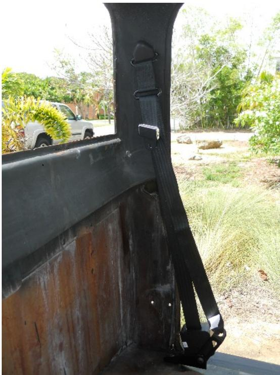
8. Once you have the retractors mounted and the shoulder loop installed you can bolt in the buckles.
