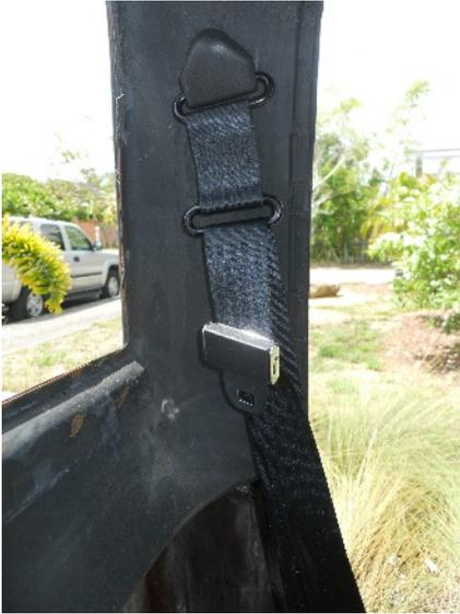
2. Most 1967-1972 Chevy trucks have the threaded shoulder belt mounting hole installed from the factory. If your truck does not have the mounting from the factory you can use the CA-53 flat plate provided with the hardware kit to make the shoulder mount. The hole should be approximately 7 inches above the bottom of the rear glass opening as seen in the photo to the left. Mark the location and move on to the next step.
