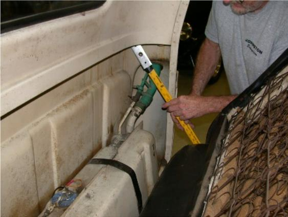
6. Install the rivets. You can now remove the bolt used to hold the plate in place.
